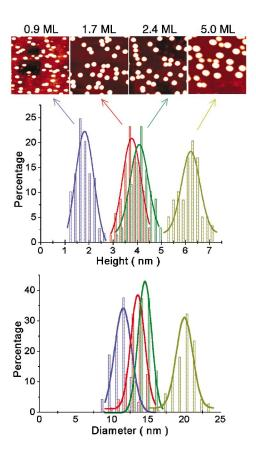
FIG. 2 (color). Typical NC-AFM images and height and diameter distributions for dots grown on NaCl(001) at different Fe coverages  $\theta$ . The image area for each coverage is 150 nm  $\times$  150 nm. The dispersions for the height distributions for the four coverages are all 0.36 nm; and the dispersions for the diameter distributions are 0.9, 1.1, 1.1, and 1.2 nm, for the four coverages, respectively.
