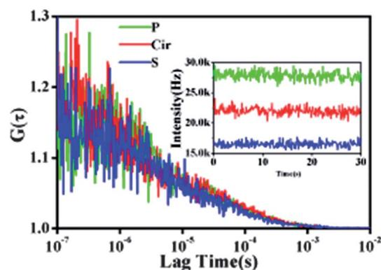
**Fig. 4** Typical ACF curves for 50 nM Cy5 solution illuminated by differently polarized light in the absence of the AuNP. The blue plot is the results for S-polarization, the red plot the results for circular polarization, and the green plot the results for P-polarization. The inset shows time traces of the fluorescence intensity measured separately for differently polarized light.
