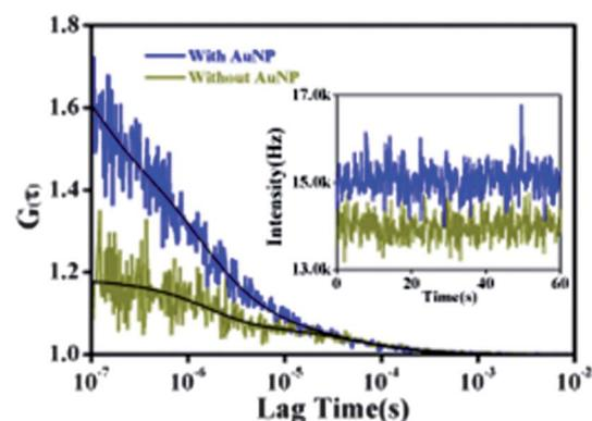
**Fig. 5** Typical TIR-FCS ACF curves measured in the presence of the AuNP (blue) and in the absence of the AuNP (brown), under S-polarized illumination. The black curves are the fitting lines obtained with eqn (3) and (5) separately. The inset shows time traces of the fluorescence intensity. The concentration of the Cy5 aqueous solution is 50 nM.
