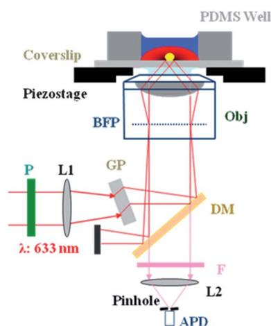
**Fig. 2** Schematic diagram of the experimental setup: P, wave plate; GP, glass plate; DM, dichroic mirror; F, fluorescence filter; L1, L2, lenses.
