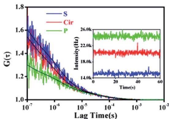
**Fig. 6** Typical TIR-FCS ACF curves measured in the presence of the AuNP with differently polarized light. The blue plot is the results for S-polarization, the red plot is the results for circular polarization, and the green plot is the results for P-polarization. The black curves are the fitting lines obtained using eqn (5). The inset shows the corresponding time traces of fluorescence intensity.
