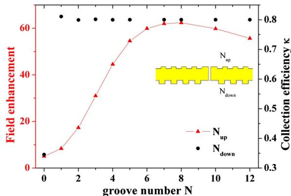
Fig. 4. Local field enhancement  $\eta_{\text{exc}}$  (red) at the slit center and collection efficiency  $\kappa$  (black) as functions of groove number  $N$  corrugated on the upper-side and bottom-side of the DG antenna. The mesh pitch here is set to be 2 nm.
