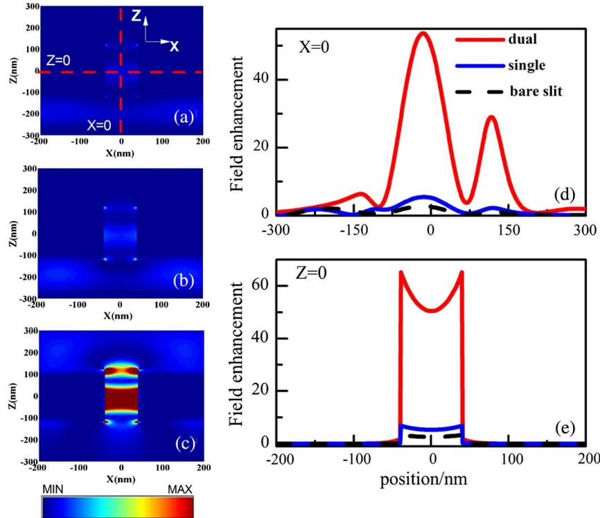
Fig. 2. Time-averaged field distributions  $|E|^2$  in the vicinity of the slit for the three metallic antennas: (a) a bare slit, (b) a SG and (c) a DG. Corresponding field enhancement factors normalized to the initial field  $|E_0|^2$  along (d)  $X = 0$  and (e)  $Z = 0$  in the  $X$ - $Z$  plane are also plotted. The structures are under normal incidence illumination with  $p$ -polarized plane wave at 633 nm.
