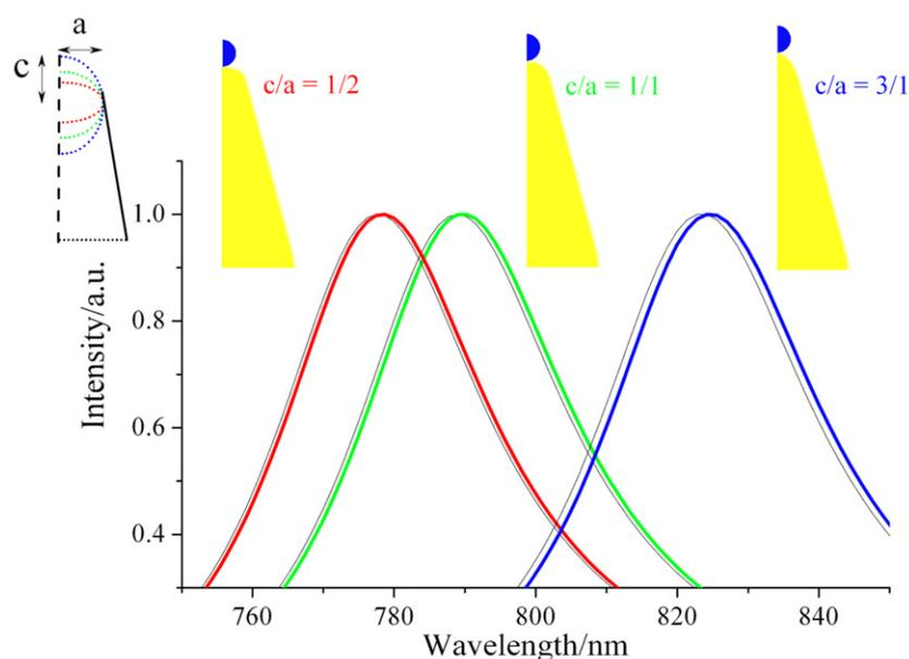
**Figure 5.** LSPR spectra of the bipyramids with different apex shape in the presence of a dielectric sphere (the LSPR spectra in the absence of the sphere are also calculated and are shown as black solid lines). The radius ratios of the different spheroid apex ends are indicated in the scheme (top left).
