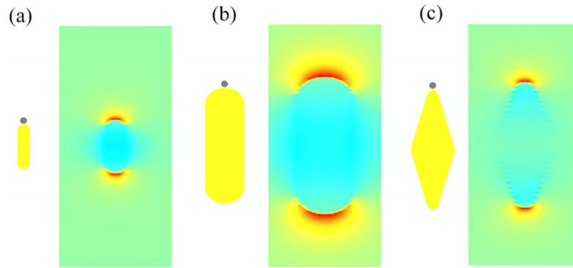
**Figure 2.** Geometrical schemes of rod-10-40, rod-30-102 and the bipyramid in the presence of a dielectric sphere and electromagnetic near-field distributions of the nanostructures illuminated with a planar continuous wave.
