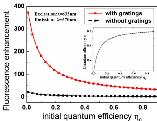
**Fig. 5** Fluorescence enhancement  $S_f/S_{f0}$  as a function of the initial quantum efficiency  $\eta_0$ .  $\eta_0$  is the quantum efficiency in solution without plasmonic antennas at 670 nm. *Inset* evolution of modified quantum efficiency  $\eta$  ( $\lambda \sim 670$  nm) versus the initial quantum efficiency  $\eta_0$
