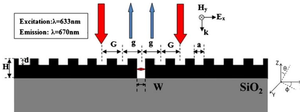
**Fig. 1** Schematic of a symmetrical slit–groove structure milled in a gold film. An electrical dipole emitter, oriented in the *x*-direction, is placed in the center of the slit. The structure is illuminated with p-polarized planar continuous light at normal incidence. Optimized
