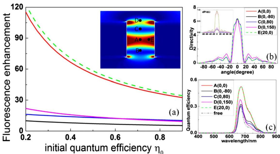
**Fig. 6** Position dependence of fluorescence characteristics for a dipole source placed in an optimized slit–groove antenna: **a** total fluorescence enhancement  $S_f/S_{f0}$ , **b** far-field directivities, and **c** quantum efficiency
