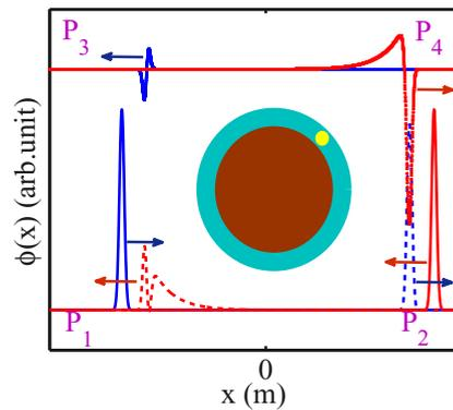
FIG. 5. (Color online) Propagation of single-photon pulses with  $\sim 4\kappa_i$  in the circulator for  $\Delta = 0$  and  $v_g = 1 \times 10^8$  m/s, as in Fig. 4. The cartoon circles indicate the cavity and the quantum impurity, respectively. The arrows indicate the moving directions. Blue (red) lines show the input and transmitted field for the left-hand (right-hand) input.
