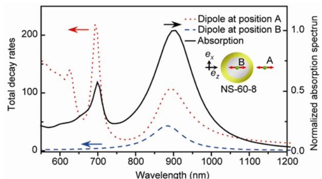
**Figure 1** (Color online) Normalized total decay rates of a point dipole source near the nanoshell with a core radius of 60 nm and shell thickness of 8 nm. The dipole is placed outside the nanoshell with a 10-nm separation (dot). The dipole is in the center of the core (dash). Normalized absorption spectrum of NS-60-8 is also shown in the black curve.
