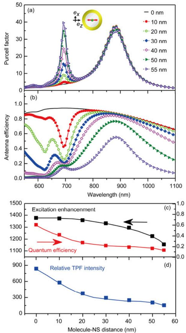
**Figure 4** (Color online) Position evolution of the Purcell Factor (a) and antenna efficiency (b) for an emitter inside coupled to the nanoshell. The distance of the emitter with the center of the core is set to 0 nm, 10 nm, 20 nm, 30 nm, 40 nm, 50 nm, and 55 nm. The two-photon excitation enhancement, quantum efficiency of Cy5.5, and relative TPF intensity as a function of the emitter NS distance are demonstrated in (c) and (d).
