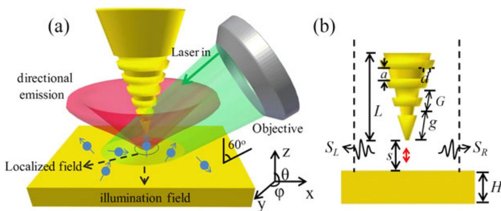
**Figure 1.** (a) Schematics of the proposed side-illumination/collection TERS configuration. A linear TM polarized beam passes through a long working distance objective with an incident angle of  $60^\circ$ . (b) Sketch of the metallic tip design:  $G=g=280$  nm,  $a=140$  nm,  $d=40$  nm,  $N=6$ . The radius of curvature at the tip end is 10 nm with an opening angle of  $30^\circ$ .
