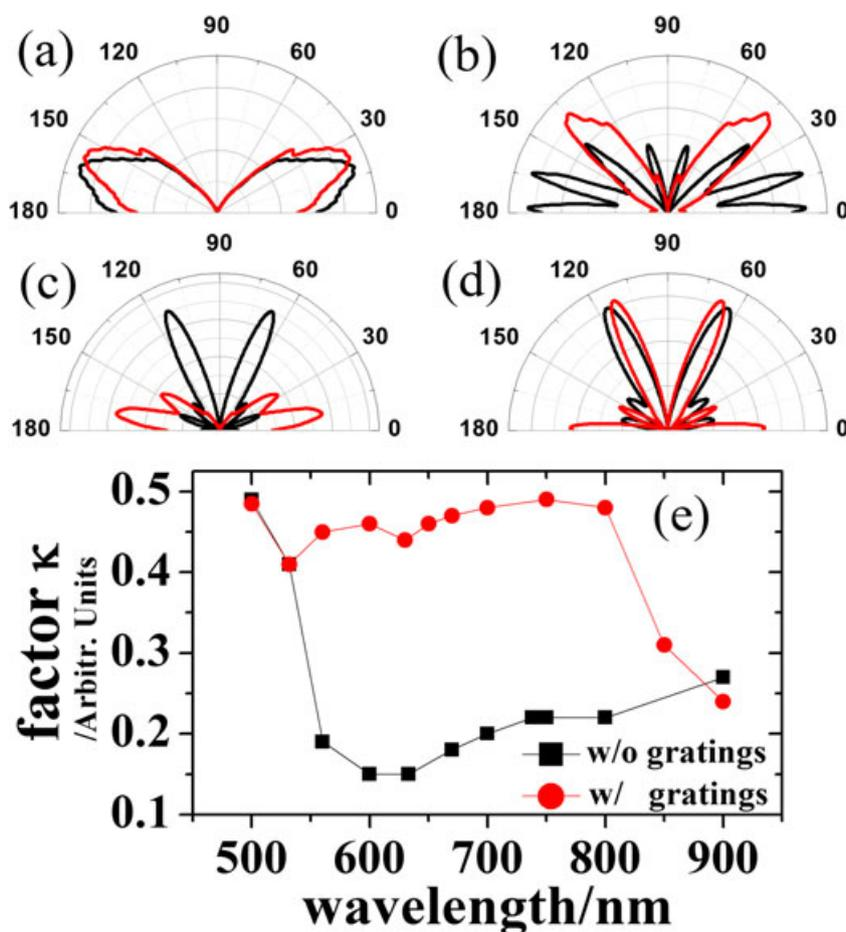
**Figure 4.** (a-d) Calculated radiation patterns for emission wavelengths at 500 nm, 532 nm, 800 nm, and 900 nm for a tip without (black) and with (red) gratings. (e) Dependence of the factor  $\kappa$  on the dipole emission wavelength. As a result of plasmonic beaming, the corrugated tip exhibits much higher collection efficiency ( $\kappa > 0.4$ ) for a wide range of wavelengths as compared with the bare tip ( $\kappa \sim 0.2$ ).
