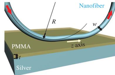
Fig. 1. Schematic diagram of the hybrid plasmonic waveguide, consisting of a bending nanofiber on a metal substrate, which is covered by a thin PMMA film (thickness  $t$ ).
