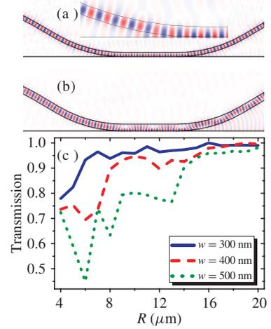
Fig. 2. (a) and (b) Filed distributions for  $w = 300$ -nm and  $w = 500$ -nm waveguide, respectively, with  $R = 10 \mu\text{m}$  and  $t = 0$ . (c) Transmission of the hybrid waveguide for different  $w$  and  $R$ , with  $t = 0$ . Inset: the detail of adiabatic conversion
