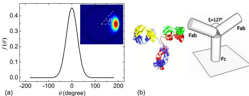
FIG. 1. (a) Mode function depending on the angle  $\theta$  defined in the inset. Inset: Cross-section mode distribution of a fundamental TE mode obtained from numerical simulation. (b) Three-dimensional structure and a simplified model of IgG antibody. The length of each rod is about 8 nm, and the diameter is 3 nm. The average angle between the two Fabs is  $127^\circ$ .
