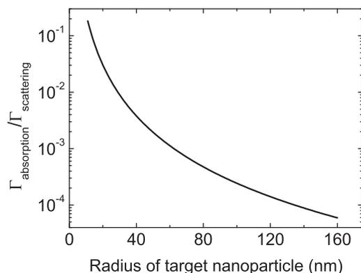
FIG. 4. Ratio of linewidth broadening induced by absorption and scattering losses depending on the radius of target nanoparticle.
