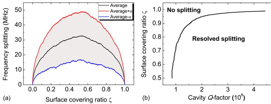
FIG. 2. (a) Frequency splitting induced by the antibody vs. the surface covering ratio  $\zeta$ , where  $\sigma$  is the standard deviation. (b) Critical cavity  $Q$ -factor for different surface coating ratio. In the upper left area of the curve, no splitting appears before adsorption of biological targets, while in the lower right area, a mode splitting is resolved after antibody coating procedure.
