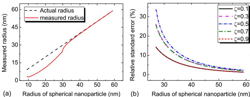
FIG. 3. (a) Measured radius of spherical nanoparticle vs. actual radius when the pre-covering ratio  $\zeta = 0.5$ . (b) Relative standard error for nanoparticle sizing depending on its radius and the different surface covering ratio  $\zeta$ .
