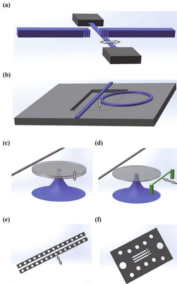
**Fig. 4** Schematics of some representative on-chip optomechanical configurations. (a) FP cavity with one of the Bragg mirrors embedded in a mechanical beam. (b) Released microring cavity coupled with substrate. (c) Double-disk cavity. (d) Microdisk coupled with a mechanical beam. (e) Photonic crystal zipper cavity. (f) Mechanical beams embedded in a photonic crystal cavity. The arrows denote the direction of mechanical oscillation.
