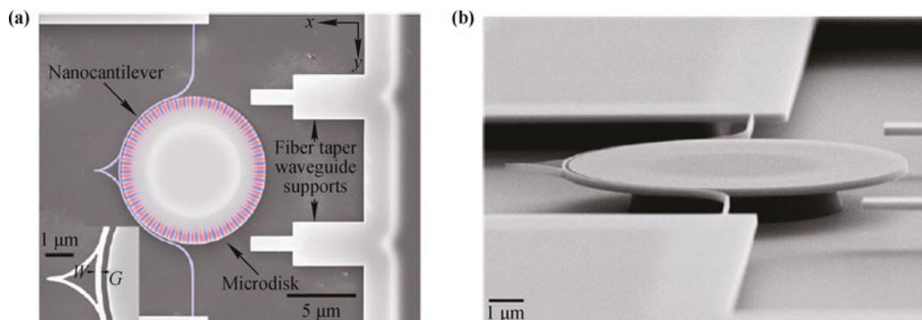
**Fig. 6** (a) Top view SEM of a bend cantilever coupled microdisk. The nano-size sharp tip in the middle of the cantilever can be used as a probe for atomic force microscope (AFM). (b) Oblique view of the same structure of the cantilever-microdisk system. Reproduced from Ref. [78], Copyright © 2011 American Chemical Society.
