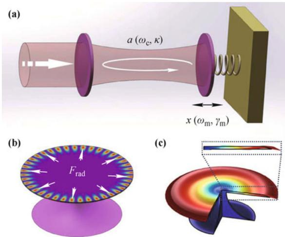
**Fig. 1** (a) Schematics of an FP cavity with a movable end mirror. (b) Illustration of a microdisk cavity and the radiation forces resulting from the circulating optical power. The calculated electromagnetic field profile is mapped on the disk. (c) Simulated fundamental radial breathing mode of the microdisk. The inset shows the cross section view of the structure deformation. Black lines denote the initial position of the boundaries.
