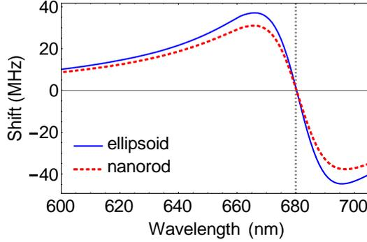
Fig. S1. Comparison of the mode shift induced by a gold ellipsoid (blue solid curve) and a gold nanorod (red dashed curve) with the same volume.
