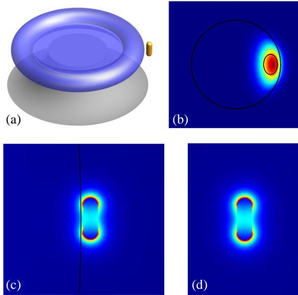
Fig. S3. 3-D FEM simulation using COMSOL. (a) Schematic setup, nanorod is at axial direction and with a 2 nm gap from the cavity surface. (b) TE fundamental mode of the cavity, the black circle represents the cavity boundary, the black ellipse inside is for finer meshing at the mode area. (c) and (d) are nanorod's electric field distribution in the azimuthal plane and the radial plane, respectively.
