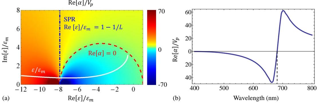
Fig. S2. (a)  $\text{Re}[\alpha]/V_p$  as a function of  $\text{Re}[\epsilon]/\epsilon_m$  and  $\text{Im}[\epsilon]/\epsilon_m$  for an ellipsoid nanoparticle. (b)  $\text{Re}[\alpha]/V_p$  as a function of wavelength when the particle material is gold.
