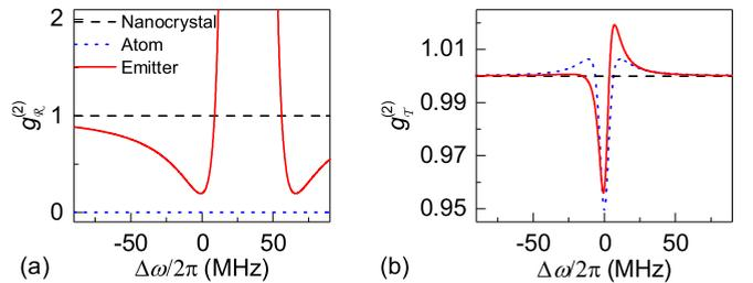
FIG. 5. Second-order autocorrelation function of the reflected field (a) and transmitted field (b). The following three different cases are plotted: (i) in the absence of the two-level artificial atom (black dashed curves); (ii) in the absence of the nanocrystal (blue dotted curves); and (iii) in the presence of both the two-level artificial atom and nanocrystal (red solid curves).
