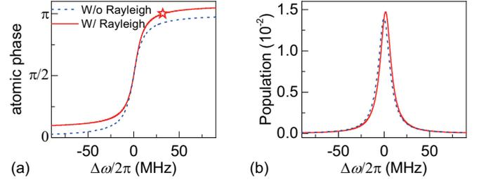
FIG. 4. Phase change of atom (a) and population of the atomic excited state (b) as a function of the detuning  $\Delta\omega$ , in the absence (blue dotted curves) and presence (red solid curves) of Rayleigh scattering. The input power is 1.5 pW. The red star indicates transparent point  $\Delta\omega = 1/\xi$ .
