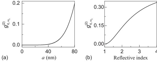
FIG. 6. Second-order autocorrelation function of reflected field of the on-resonance incident optical field  $\omega = \omega_0$  as a function of the radius  $a$  (a) and refractive index (b) of a nanocrystal.
