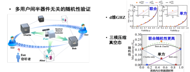
图 1: 多用户量子网络中半器件无关的随机数验证方案 (左图), 基于多方联合测量结果可以比基于单方的方案验证更高的随机性, 且方案适用于任意维度系统 (右图)。FIG. 1. Schematic view on randomness generation in multipartite network (Left). A controller sends a tripartite state \rho_{ABC} to three nodes. Two of these nodes (Bob and Charlie) perform measurements with the aim to use the results as a source of randomness.
