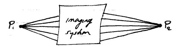
Thus, according to Fermat's Principle, <u>all</u> the rays from  $P_1$  to  $P_2$  must travel <u>exactly the same path length</u>. (And they are all, of course, the minimum path length.)
