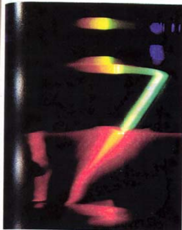
FIGURE 2-11. Propagation of light in an absorbing medium. Light from a HeCd laser propagates through first a layer of xylene and then water containing the dye, Rhodamine 6G, in solution. The blue laser light is absorbed by the Rhodamine as the wave propagates through the water. The Rhodamine reemits the energy in the form of a red fluorescence. The reemitted light is radiated in all directions, making the beam appear diffuse. Some of the absorbed energy is not reemitted but instead heats the Rhodamine.
