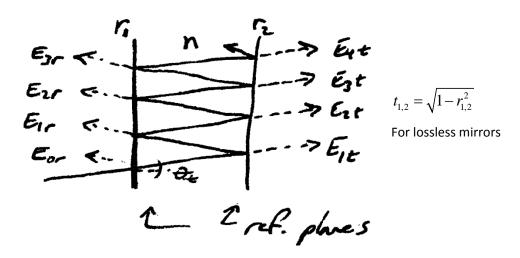
The calculation of the transmitted and reflected waves is straightforward: just add up all the "partial waves"
