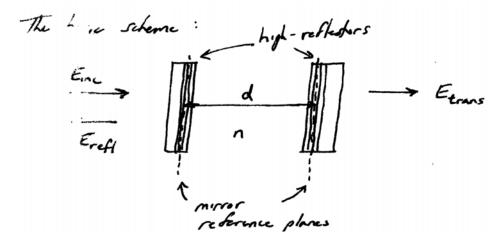
Since the mirrors are high reflectors, we can no longer consider only one reflection at each mirror as we did in the dielectric slab problem; we must involve <u>all</u> the reflections.
