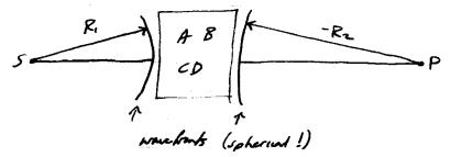
The ABCD matrix transforms the ray angles and displacements such that S and P are conjugate. It is also interesting (and will turn out to be extremely useful in the context of Gaussian beams!) to consider the effect of the element ABCD on the wavefront.
