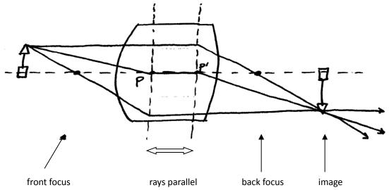
note: rays through principal points P and p' are still parallel outside the lens (as long as n is the same on both sides , as we have been assuming).
