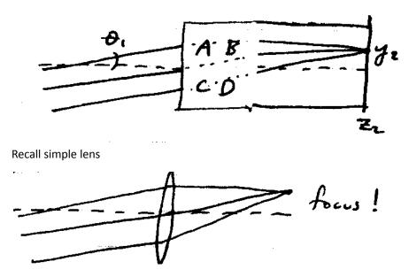
Thus if <u>A=0</u>, the second reference plane of the ABCD system must be the <u>second focal plane</u> of the system!
