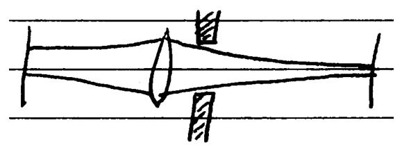
For a temporal imaging system, this is generally not the case. The aperture is not really something that prevents light from getting through if it's not within the aperture
