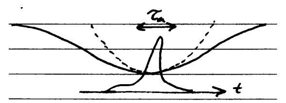
Thus components of the pulse outside  $\tau_m$  will not be neglected, but will be distorted in time(i.e. higher-order phase errors, leading to wings on the pulse)
